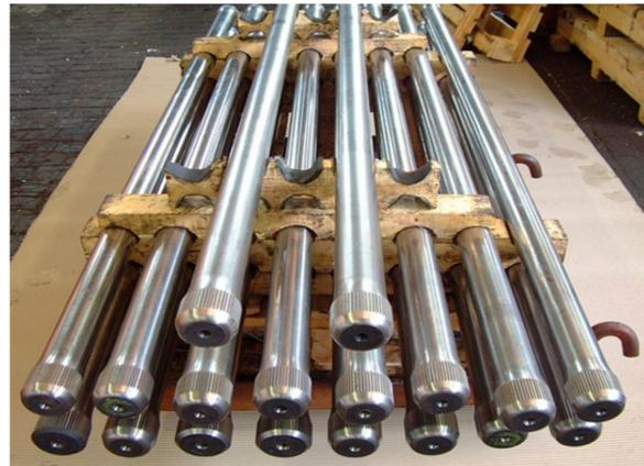
**Figure 1.** Set of torsion spring bars ready for delivery.
