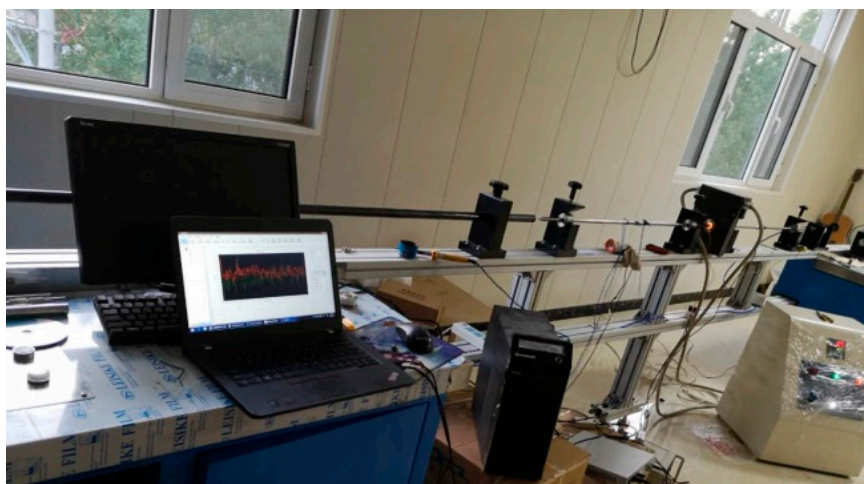
Figure 2. Device diagram of split Hopkinson pressure bar experiment.
