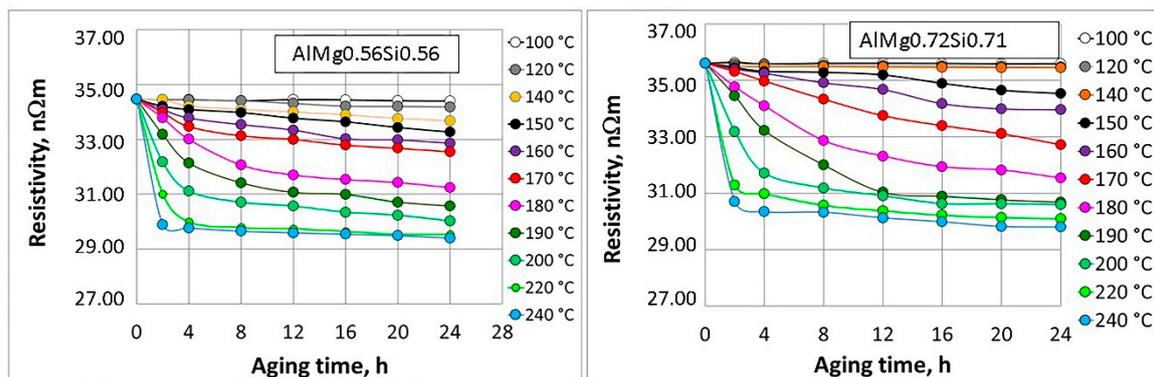
Figure 6. Relationship between resistivity and artificial aging time at different temperatures for the AlMg0.56Si0.56 and AlMg0.72Si0.71 wire rods.
