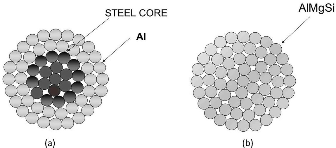
**Figure 1.** Aluminum conductor steel reinforced (ACSR) (a) and all aluminum alloy conductors (AAACs) (b).
