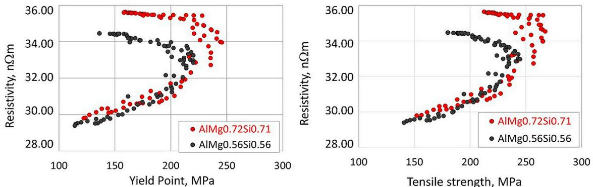
**Figure 8.** Relationship between the yield point and resistivity and between the tensile strength and resistivity of Al-Mg-Si wire rods after artificial aging (black points: AlMg0.56Si0.56, red dots: AlMg0.72Si0.71).
