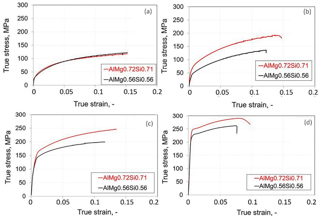
**Figure 3.** True stress and true strain curves of Al-Mg-Si wire rods with different amounts of Mg and Si after homogenization (a), supersaturation (b), natural aging (c) and artificial aging (d).
