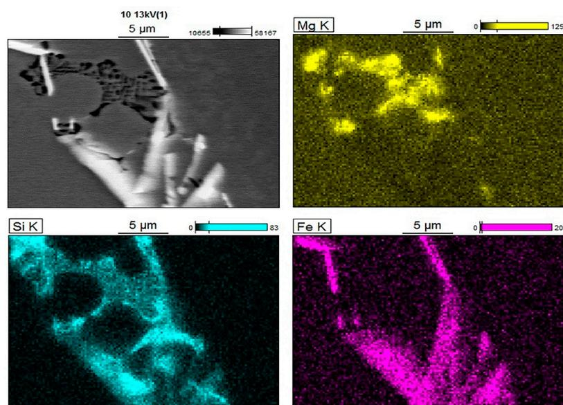
**Figure 4.** EDS analysis of the AlMg0.72Si0.71 wire rods after homogenization.
