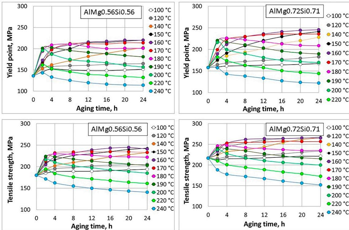
**Figure 7.** Relationship between strength and artificial aging time at different temperatures for the AlMg0.56Si0.56 and AlMg0.72Si0.71 wire rods.
