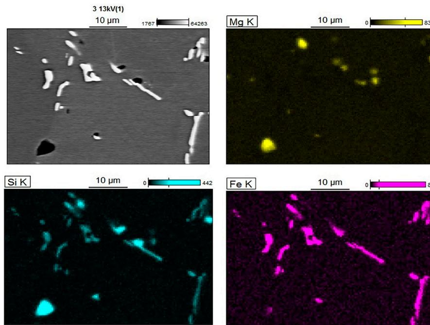
Figure 5. EDS analysis of the AlMg0.56Si0.56 wire rods after homogenization.
