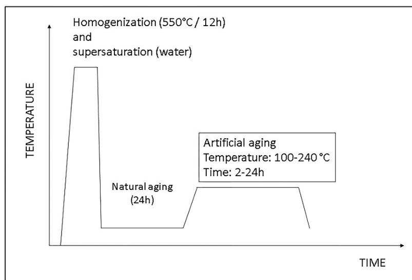
**Figure 2.** Scheme of the heat treatment of the wire rods.
