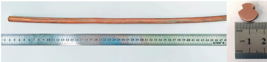
**Figure 9.** General view of the experimental samples of contact wire from the Cu–0.5Cr alloy produced by combined processing.
