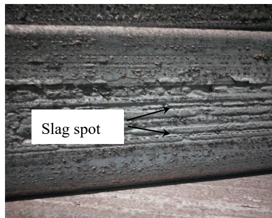
Figure 1. Typical SWRH82B billet surface slag spots.
