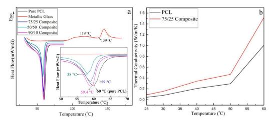
**Figure 2.** DSC thermographs for (**a**)  $Mg_{66}Zn_{30}Ca_4$  metallic glass, pure PCL, and different metallic glass/PCL composites; (**b**) thermal conductivity of the pure PCL and 75/25 composite samples. The melting points of the pure PCL and composites samples under higher magnification in the insert.
