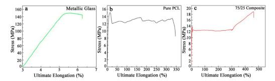
**Figure 1.** Tensile engineering stress-strain curves for (**a**)  $Mg_{66}Zn_{30}Ca_4$  glassy ribbon, (**b**) pure polycaprolactone, and (**c**)  $Mg_{66}Zn_{30}Ca_4/PCL$  75/25 composite.
