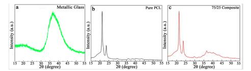
**Figure 3.** X-ray diffraction patterns of the (**a**) metallic glass, (**b**) PCL, and (**c**) Mg<sub>66</sub>Zn<sub>30</sub>Ca<sub>4</sub>/PCL 75/25 composite.
