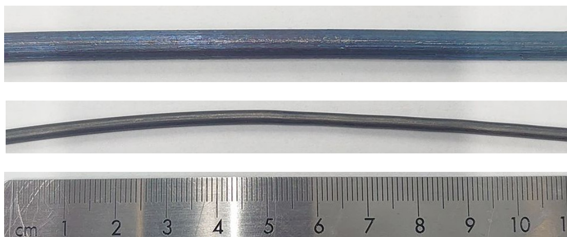
Figure 6. Photograph of as-Conformed CP-Ti Gr 2 wire with blue oxide film ( top ) and \varnothing 3.00 mm cold-wire-drawn wire with bright surface ( bottom ) from the same extruded product.
