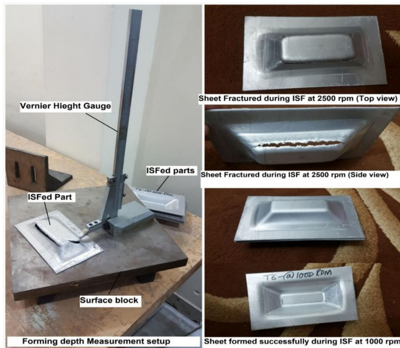
Figure 5. Setup showing measurement of forming depth and representatives of successful and unsuccessful samples.
