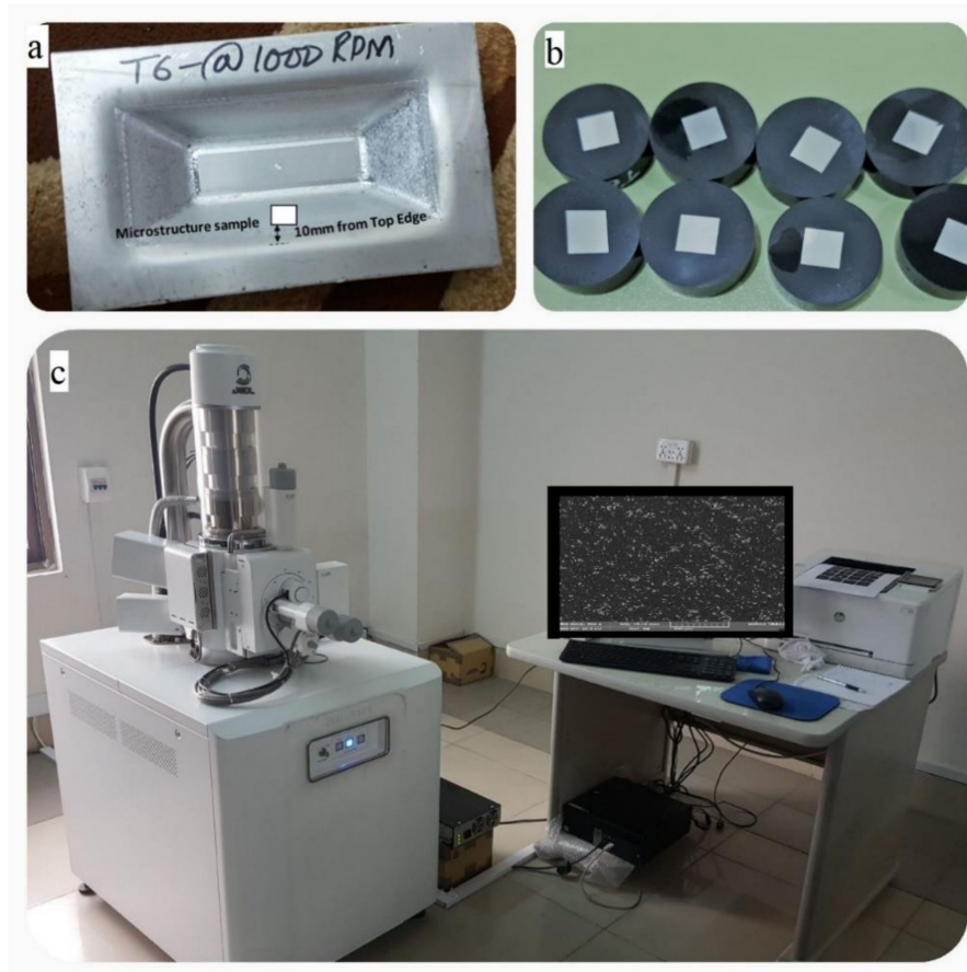
Figure 3. Metallography details: (a) sample extraction, (b) molded metallography samples and (c) scanning electron microscope (Model: IT100LA, JEOL Ltd. Tokyo, Japan).
