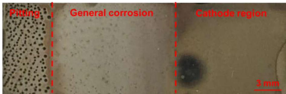
**Figure 4.** Appearance of the 30 mm long BPE after bipolar electrochemistry testing for 30 min, with the left side showing large pits at the oxidation edge and the right side showing the reduction edge.
