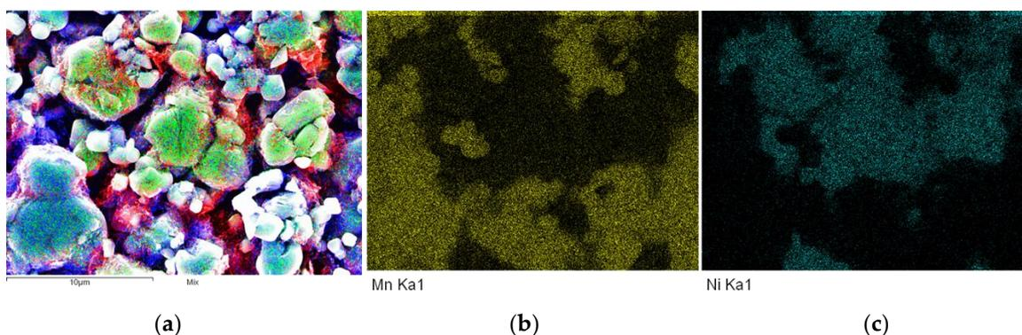
**Figure S1. 1** EDX mapping analysis showing distribution of the elements (a), the transition metals Mn (b) and Ni (c) in the SEM images, there appear to be two separate phases the first is Mn rich, the second is Ni rich.
