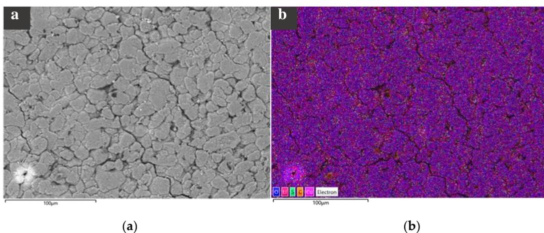
**Figure S2. 1** SEM (a) and EDS elemental mapping (b) of QC rejected anode, showing copper contamination throughout the electrode.
