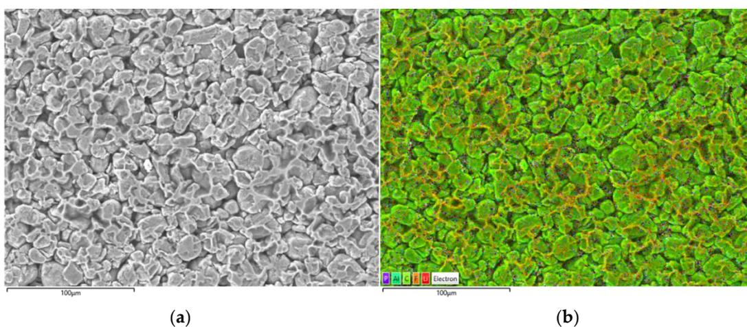
**Figure S2. 2** SEM (a) and EDS elemental mapping (b) of EOL cell, showing carbon particles and patches of high fluorine content due to the PVDF binder.
