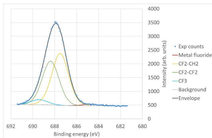
**Figure S2. 3** XPS analysis of the surface of the QC rejected anode black mass, and the fluorine analysis.
