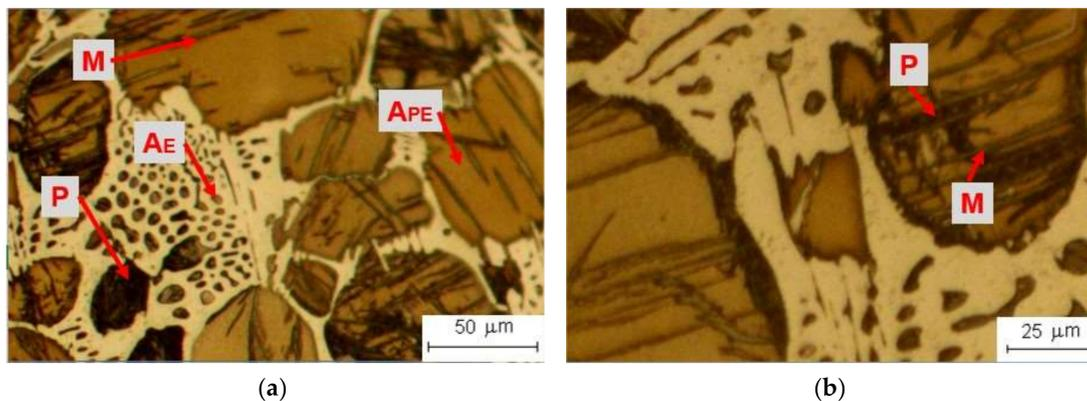
**Figure 11.** Picral reagent: (a) general view at 200×; (b) detail at 500×.
