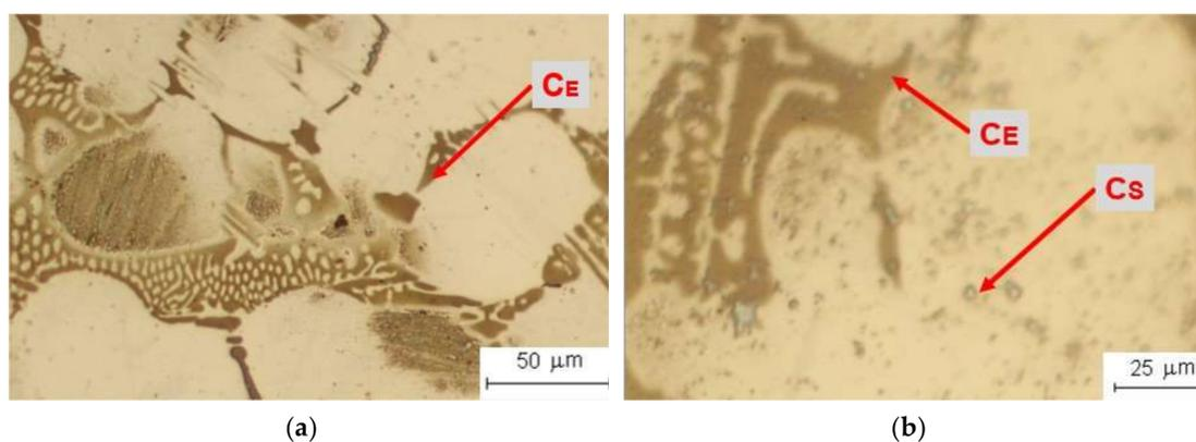
**Figure 7.** Murakami reagent at room temperature: (a) general view at 200 $\times$ ; (b) detail at 500 $\times$ .
