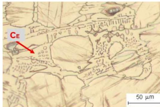
**Figure 1.** Marshall reagent for 5 s at room temperature (200×).
