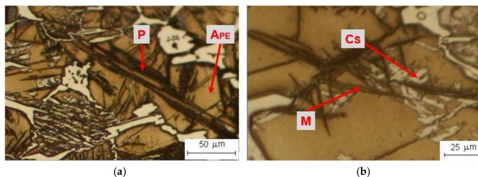
**Figure 5.** Attack 4 (Marshall reagent for 60 s at room temperature, 5% ammonium persulfate at room temperature) + Kalling N°1: (a) general view at 200 $\times$ ; (b) detail at 500 $\times$ .
