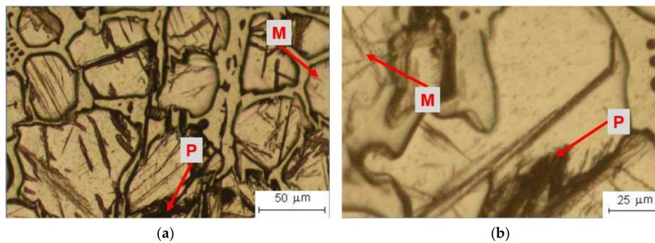
**Figure 3.** Marshall reagent for 60 s at room temperature: (a) general view at 200 $\times$ ; (b) detail at 500 $\times$ .
