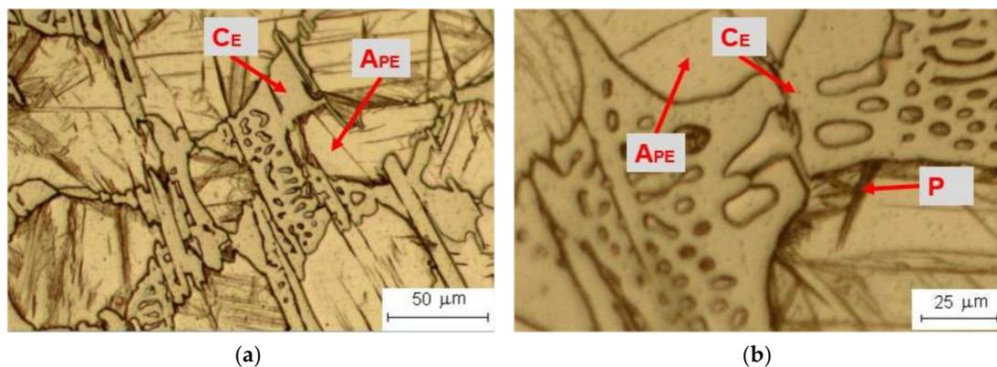
**Figure 2.** Marshall reagent for 25 s at room temperature: (a) general view at 200×;(b) detail at 500×.
