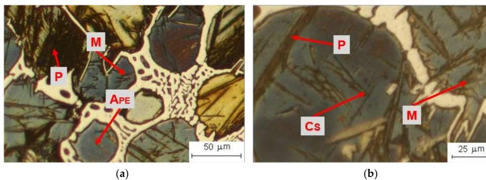
**Figure 4.** Attack 3 (Marshall reagent for 60 s at room temperature) + 5% ammonium persulfate at room temperature: (a): general view at 200 $\times$ ; (b) detail at 500 $\times$ .
