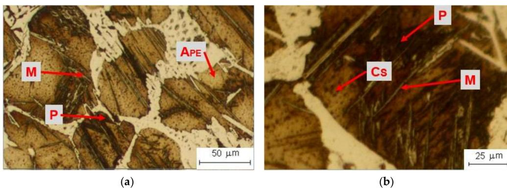
**Figure 10.** Marble reagent at room temperature: (a) general view at 200×; (b) detail at 500×.
