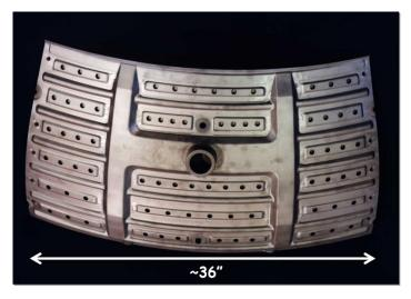
**Figure 3.** Example of a complex sheet metal engine part made by superplastic forming and diffusion bonding (SPFDB) [2].
