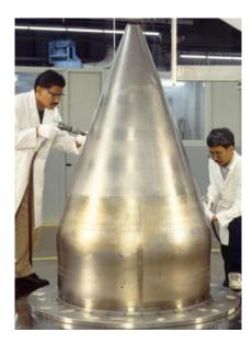
**Figure 11.** Fabricating the  $\beta$ -21s tail plug for the B-777 engine.
