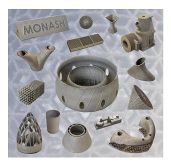
**Figure 4.** Examples of parts with complex geometries made by powder bed AM. Figure courtesy of Prof. Xinhua Wu, Monash University, Melbourne, Australia.
