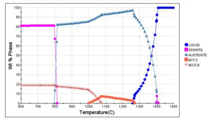
**Figure 1.** Phase equilibrium diagram of 440C martensitic stainless steel, obtained from JMatPro<sup>®</sup> simulation software.
