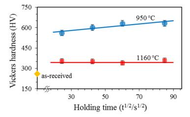
Figure 6. Effect of PS treatment holding time on the hardness of samples.
