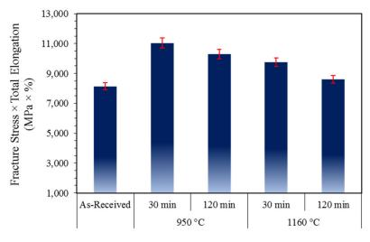
Figure 9. Strength-ductility balance of samples heat-treated for 30 and 120 min.
