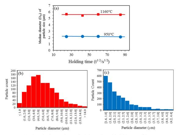
**Figure 5.** (**a**) Relationship between the size of carbide particles and the holding time of the PS treatment. (**b**) Histograms of particle size measurement of 1160-sample and (**c**) 950-sample treated for 30 min.
