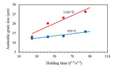
**Figure 4.** Relationship between the austenite grain size of 1160 sample and 950-sample and the holding time during the PS treatment.
