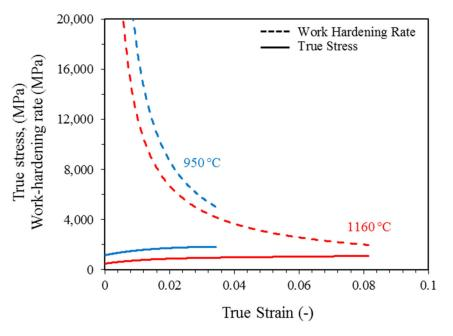
Figure 10. True stress and work-hardening rate of 1160-sample and 950-sample, heat treated for 30 min.
