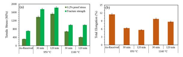
**Figure 8.** Tensile properties of samples heat-treated for 30 and 120 min: (**a**) yield and fracture stresses and (**b**) total elongation.
