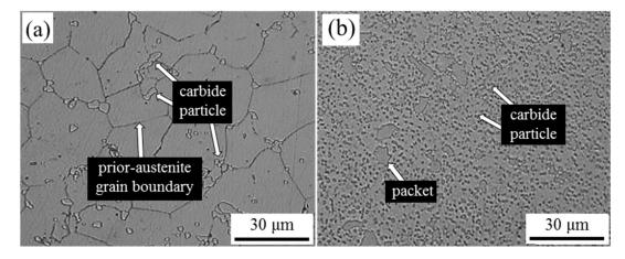
**Figure 2.** Optical micrographs: (**a**) 1160-sample and (**b**) 950-sample with the holding time of 30 min for the partial solution (PS) treatment.
