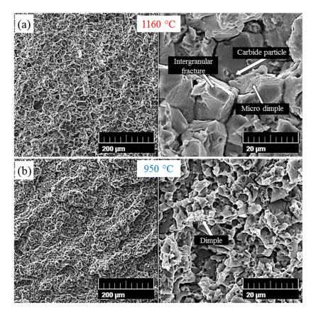
Figure 12. SEM images of fracture surface: (a) 1160-sample and (b) 950-sample, at different magnifications.
