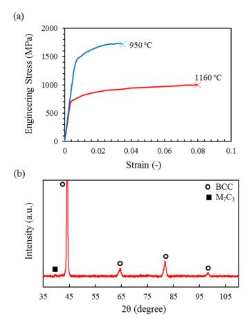
**Figure 7.** (a) Engineering stress-strain curve of samples treated for 30 min and (b) XRD diffractograms of tensile-tested 1160-sample.
