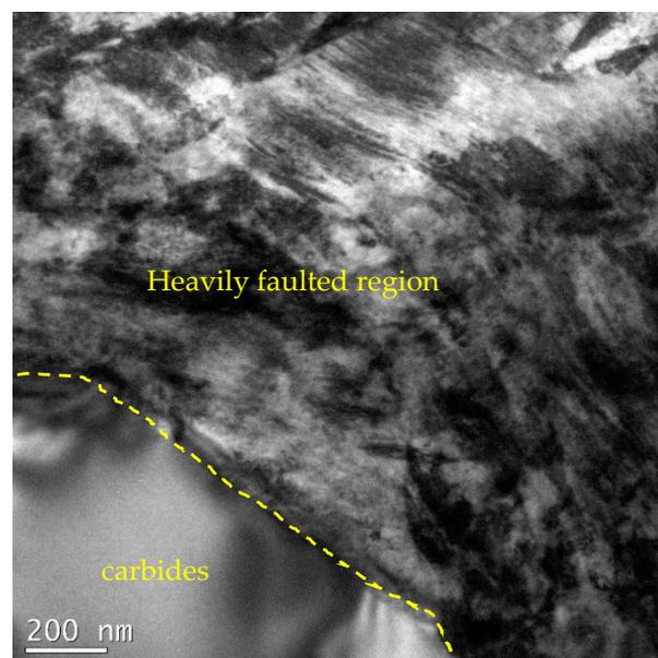
**Figure 4.** High-resolution TEM image showing the heavily faulted region at the carbide/matrix interface.
