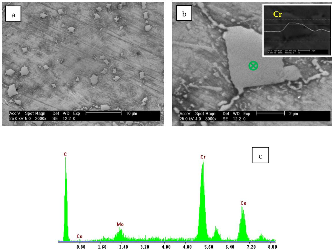
**Figure 1.** SEM micrographs of (a) the partial solution sample and (b) undissolved primary carbides. (c) EDS point analysis of the precipitated carbide.
