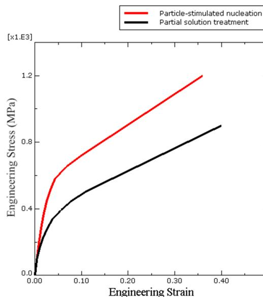
**Figure 5.** Engineering stress–strain curves of specimens after partial solution treatment (black curve) and particle-stimulated nucleation of recrystallization (red curve) at  $850 \text{ }^\circ\text{C}$  for 30 min.
