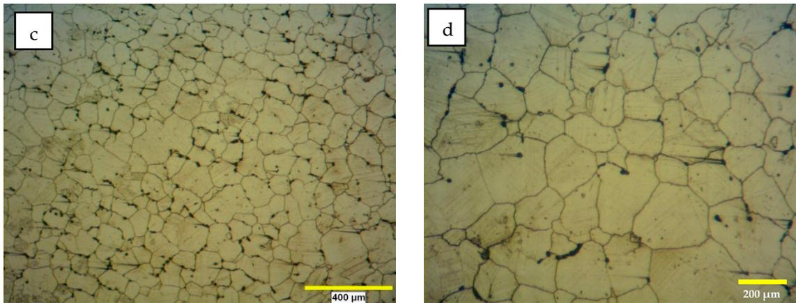
**Figure 2.** (a–d) Optical micrographs of the fine recrystallized grains nucleated in the vicinity of carbide particles for 15 and 30 min, respectively.
