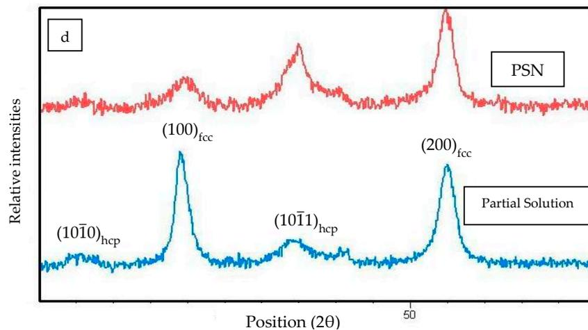
**Figure 3.** (a,b) Particle-stimulated nucleation of recrystallization at carbides. (c) Recrystallization originates from the deformation zone near the carbides. (d) XRD graphs of the partial solution and particle-stimulated nucleation (PSN) specimens.
