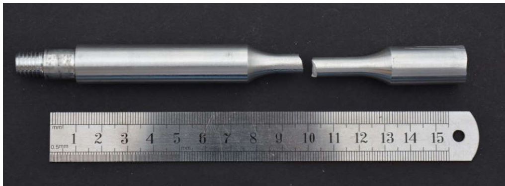
Figure 11. Rotating bar bending test fractured.
