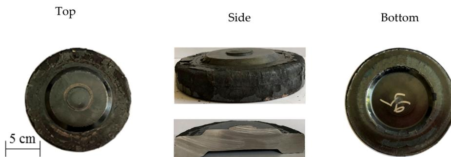
**Figure 4.** Specimen with  $ZrO_2$  content of 5%.
