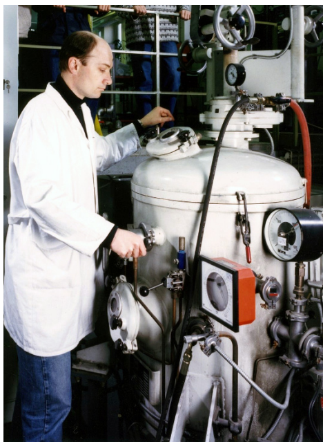
Figure S1-2. Vacuum induction-melting furnace; the continuous caster is placed below the furnace but cannot be seen.
