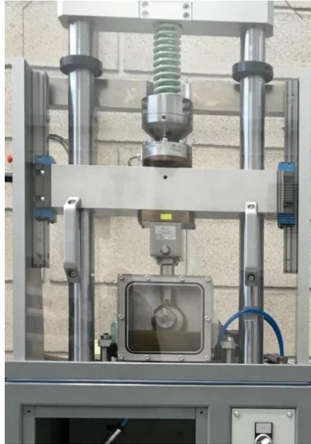
**Figure 3.** Equipment for testing the in-service wear behaviour of mechanical parts.
