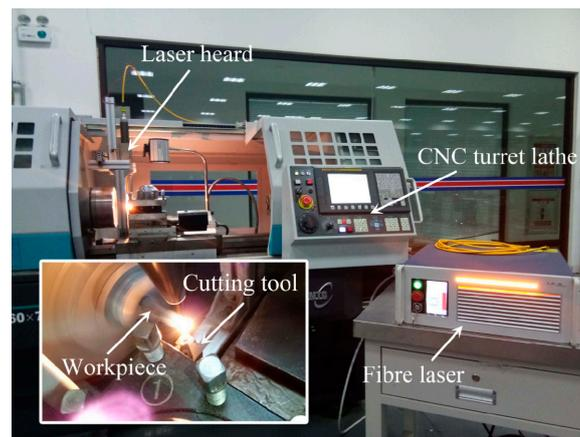
**Figure 1.** Experimental system for LAM of silicon nitride.
