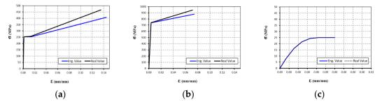
Figure 3. Constitutive models considered for (a) ASTM-A36 steel, (b) ASTM-A193 steel and (c) concrete.
