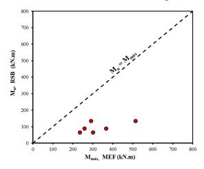
Figure 9. Comparison of FEM results with estimations of the rectangular stress block (RSB) method.
