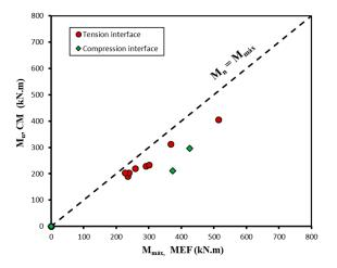
Figure 10. Comparison of FEM results with estimations of the component method (CM).
