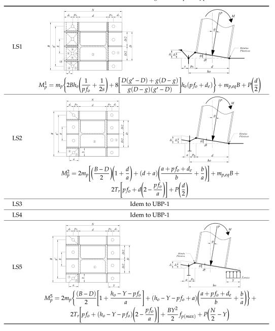
Table 4. Limit states that control the design of base plate type SBP-1.
