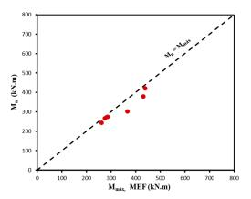
**Figure 12.** Comparison of flexural strength estimations of the proposed method with FE models results for stiffened base plates.
