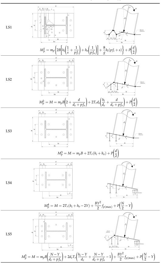
Table 3. Limit states that control the design of base plate type UBP-2.
