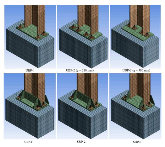
Figure 2. Finite element models for each specimen configuration.
