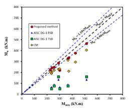
**Figure 11.** Comparison of flexural strength estimations of the different methods with FEM results for non-stiffened base plates.
