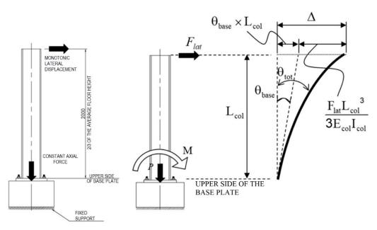
Figure 4. Loading protocol and response parameters.
