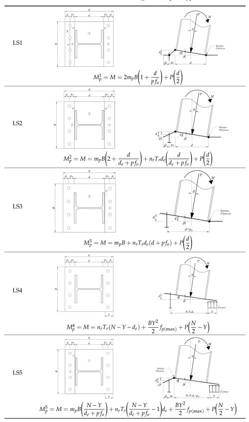
Table 2. Limit states that control the design of base plate type UBP-1.
