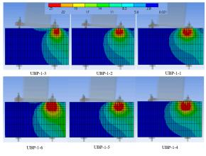
(e) Von-Mises stress distribution in concrete (MPa).
