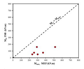
Figure 8. Comparison of FEM results with estimations of the triangular stress block (TSB) method.
