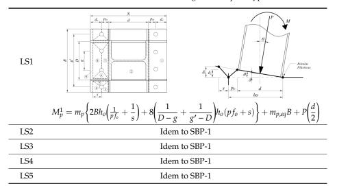
Table 5. Limit states that control the design of base plate type SBP-2.
