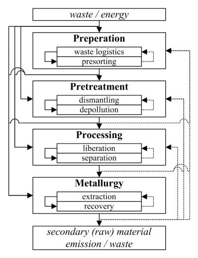
Figure 1. Recycling chain with process stages and unit processes for spent lithium-ion batteries.
