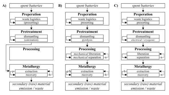
**Figure 6.** Schematic flow chart of the three most common industrial process routes: high temperature route (**A**), moderate temperature route, (**B**) and low temperature route (**C**); p—pyrometallurgical, h—hydrometallurgical, n—number of iterations.
