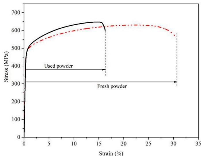
**Figure 10.** Stress-strain curves of AISI 316L produced by DED using fresh and recycled powders [136].
