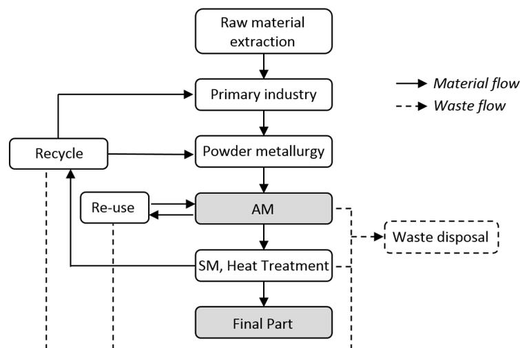
Figure 7. Material product life cycle in AM. Adapted from [107].
