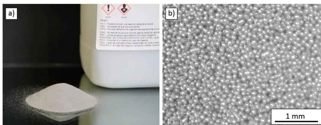
**Figure 4.** (a) AISI 316L powder and container with the hazard details, (b) AISI 316L.
