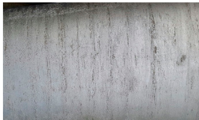
Figure 3. Sand side of cast sheet with grooves (1000 mm × 600 mm).
