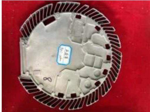
**Figure 11.** 6063 Al telecom part fabricated by the RheoMetal [130].
