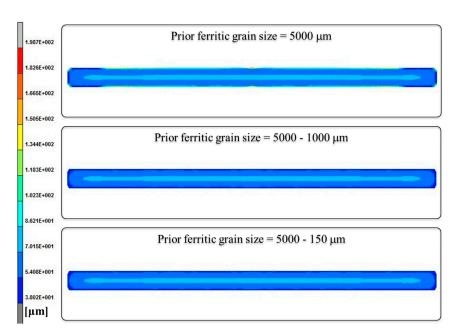
Figure 12. Effect of different PFGS on the ferrite grain size after the fifth roughing pass.
