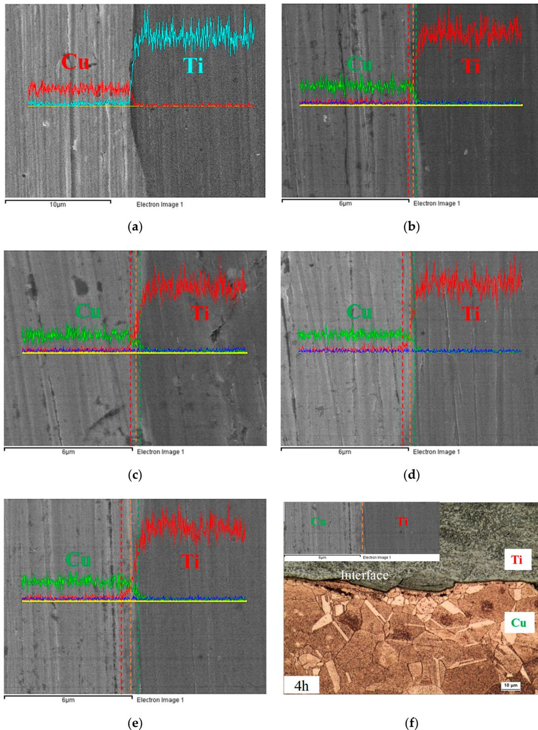
**Figure 1.** Line scanning analysis results of titanium clad materials: (a) as-rolled sample and samples annealed at 450 °C for (b) 0.5 h, (c) 1 h, (d) 2 h, (e) 4 h, and (f) interfacial microstructure for 4 h.
