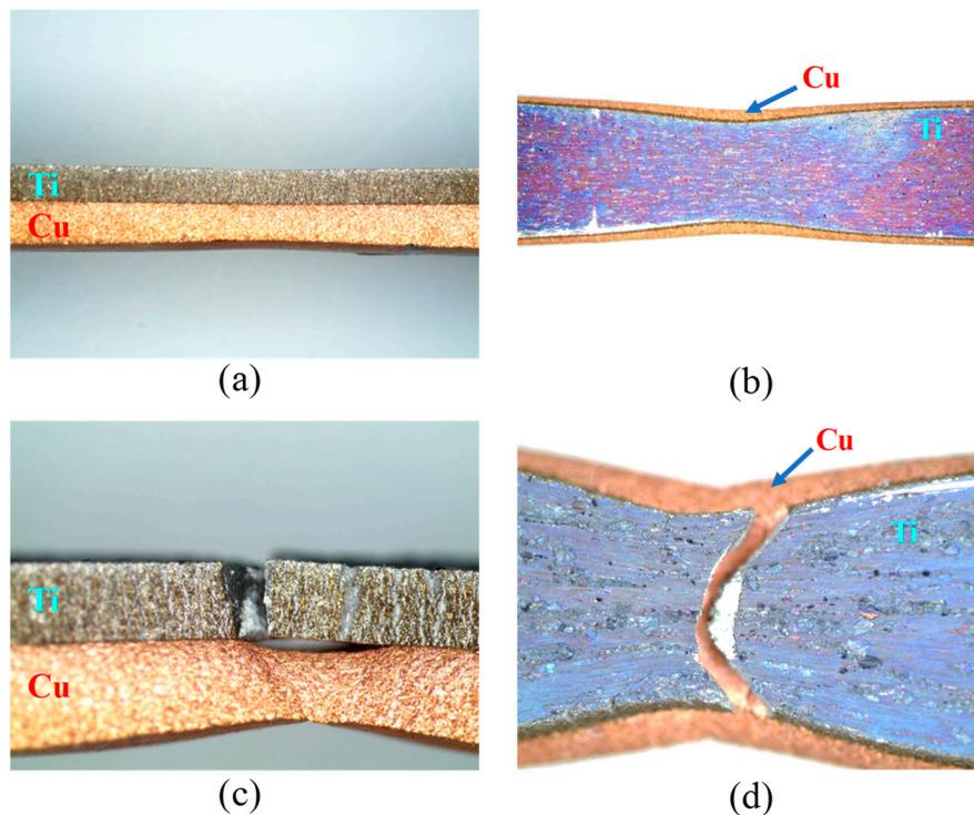
**Figure 6.** Top-view and side-view of the titanium clad during the tensile test: (a,b) 1 h and (c,d) 2 h; (a,c) side-view and (b,d) top-view.
