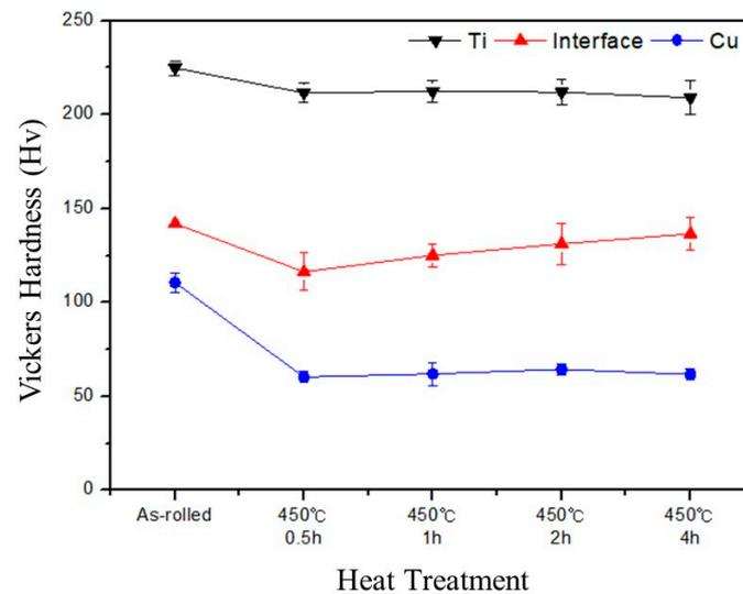
**Figure 4.** Vickers micro hardness of the component layers (Ti, Cu) and interface layers (Ti/Cu) for as-rolled and annealed clads.
