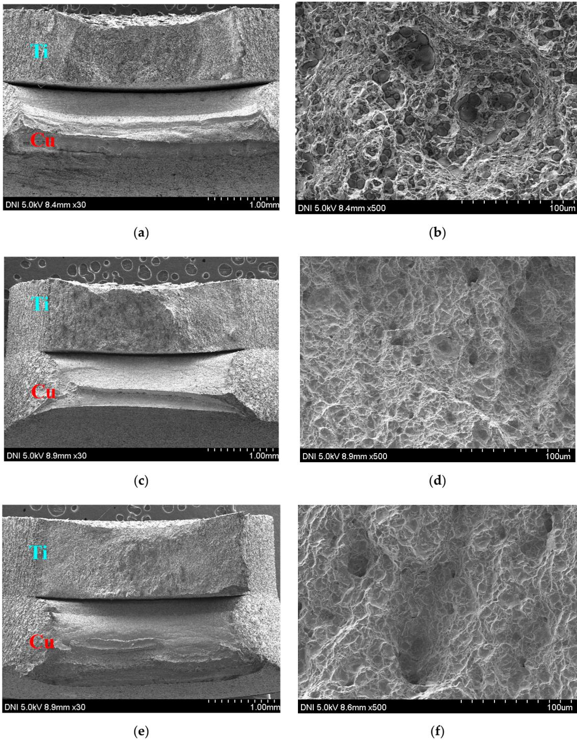
**Figure 7.** SEM images of fracture surfaces: (a,b) as-rolled sample; samples annealed at 450 °C for (c,d) 2 h and (e,f) 4 h.
