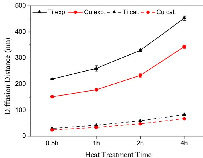
**Figure 2.** Experimental and theoretical values of diffusion distance.
