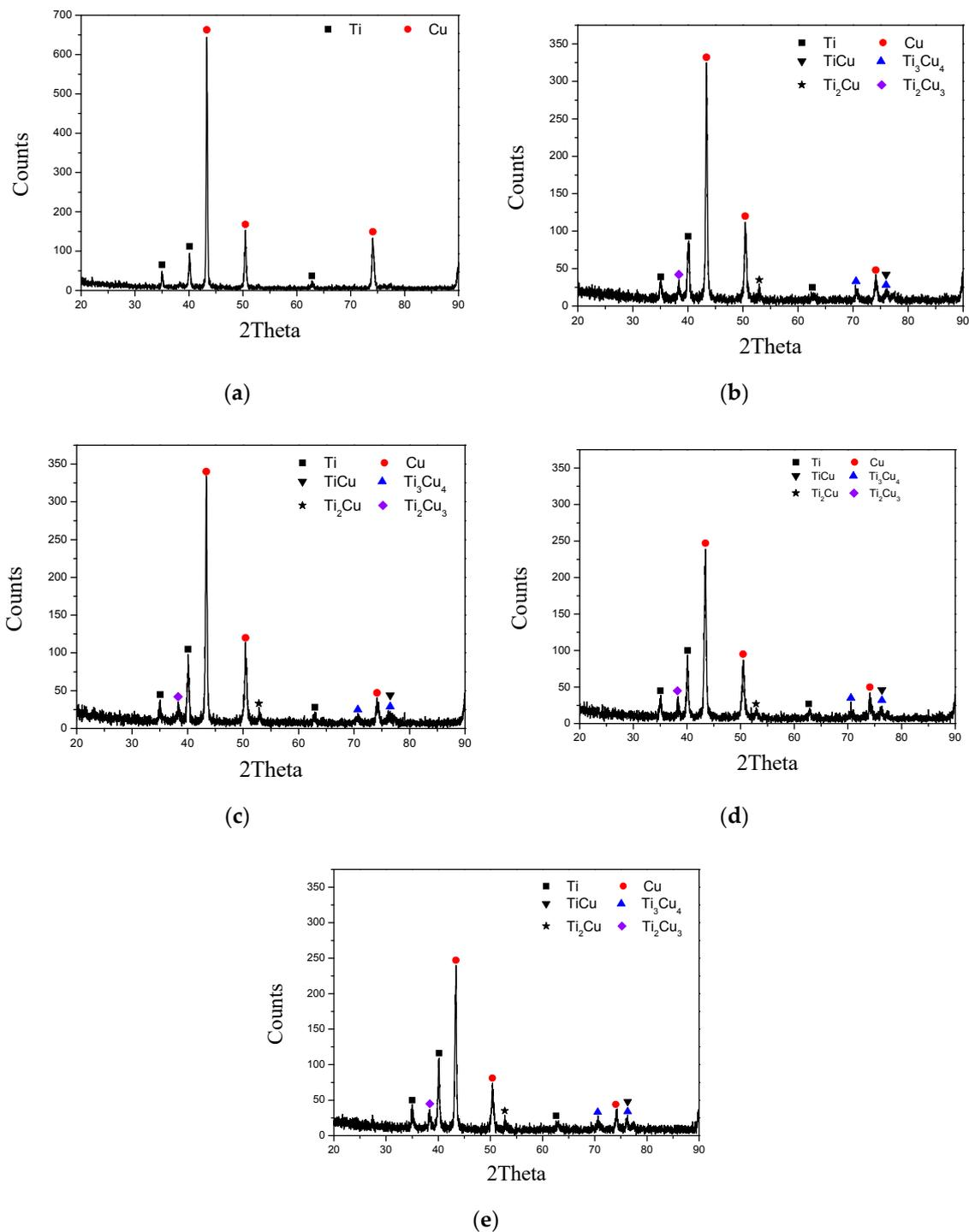
**Figure 3.** XRD patterns of titanium clad materials: (a) as-rolled sample, and samples annealed at 450 °C for (b) 0.5 h, (c) 1 h, (d) 2 h, and (e) 4 h.
