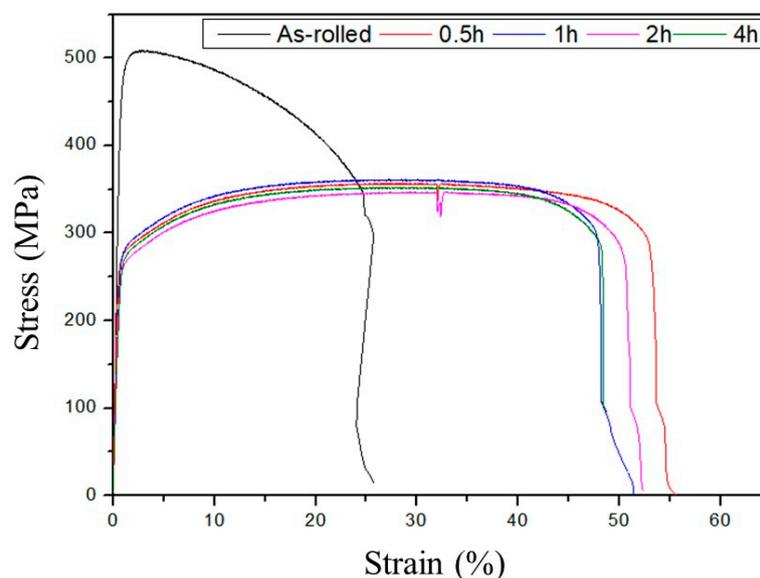
**Figure 5.** Stress–strain responses of as-roll-bonded clad metals annealed at 450 °C for different times.
