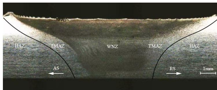
Figure 3. Cross-sectional morphology of the friction stir welded (FSW) joint.
