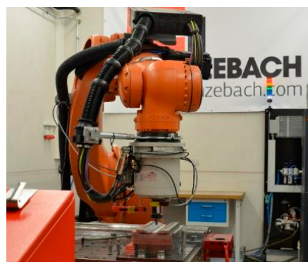
Figure 2. Robotized FSW setup and clamping structure.
