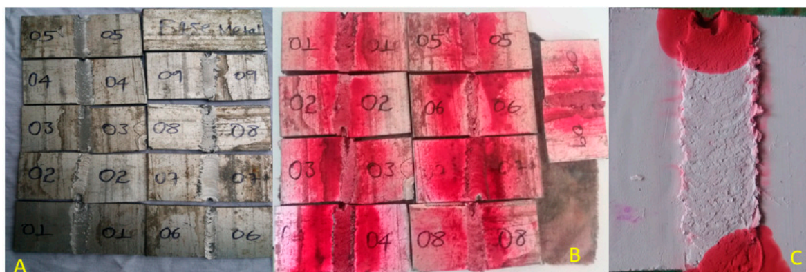
Figure 8. Liquid penetrant test: (A) Welded specimens before the liquid penetrant test; (B) welded specimens after applying penetrants on the faying surfaces; (C) welded specimens after applying developer.
