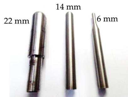
**Figure 3.** Hemispherical head high-speed steel (HSS) tools.
