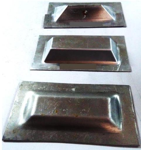
**Figure 4.** Pyramid frusta produced via the SPIF.
