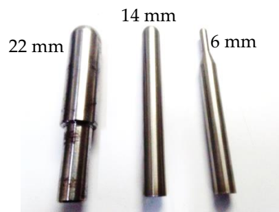
Figure 3. Hemispherical head high-speed steel (HSS) tools.
