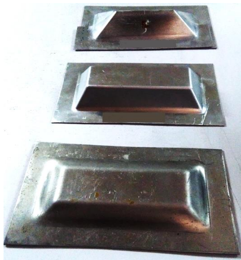
Figure 4. Pyramid frusta produced via the SPIF.
