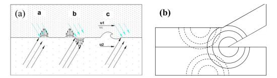
**Figure 10.** (a) Helmholz instability mechanism (reproduced from [37], with permission of Elsevier 2010); (b) stress wave mechanism.
