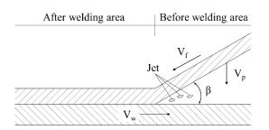
Figure 5. Schematic diagram of the impact welding process.
