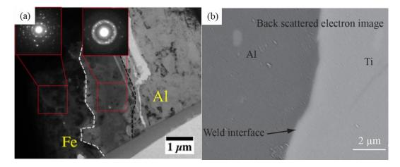
**Figure 12.** Two welding interfaces of impact welding (**a**) Transition zone interface (reproduced from [49], with permission of Elsevier 2019); (**b**) Interface without transition zone (reproduced from [24], with permission of Laser Institute of America 2016).
