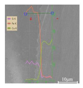
Figure 14. EDS concentration curve for laser impact welding of crystal and amorphous materials [52].
