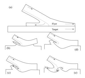
**Figure 9.** (**a**–**e**) the process of Bahrani caved mechanism (reproduce from [34], with permission of Royal Society 1967).
