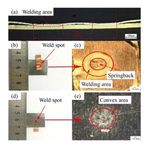
**Figure 7.** (a) Cross-section of weld interface at 1550 mJ energy (reproduced from [27], with permission of Elsevier 2019); (b–e) Weld spot between molybdenum and copper (reproduced from [28], with permission of Elsevier 2019).
