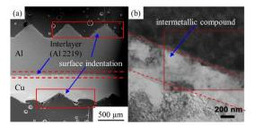
**Figure 1.** (a) Surface indentation of ultrasonic welding (reproduced from [9], with permission of Elsevier 2020); (b) Intermetallic compound layer with friction stir welding (reproduced from [15], with permission of Elsevier 2015).
