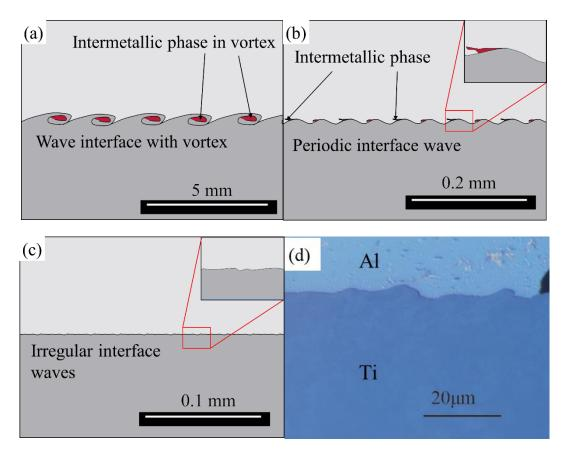
**Figure 8.** Weld interface morphology of three typical impact welded joints with (**a**) Explosive welding; (**b**) Magnetic pulse welding; (**c**) Laser impact welding; (**d**) Weld wave interface morphology with laser impact welding (reproduced from [24], with permission of Laser Institute of America 2016).
