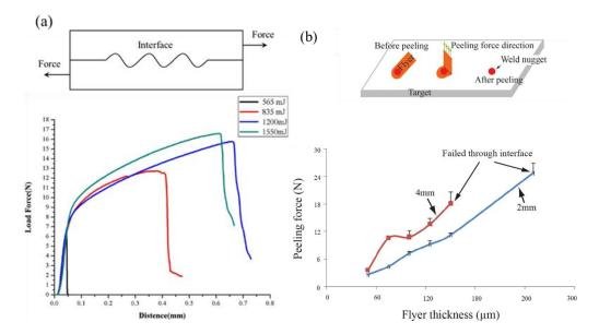
**Figure 15.** Test method for bonding force of welded joints (**a**) shearing test and result (reproduced from [28], with permission of Elsevier 2019); (**b**) peeling test and result (reproduced from [24] with permission of Laser Institute of America 2016).
