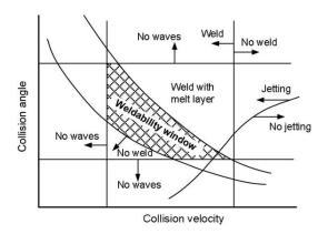
Figure 6. Generic welding window (reproduced from [10], with permission of Elsevier 2019).
