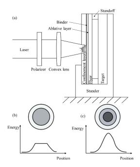
**Figure 3.** (a) Schematic diagram of laser impact welding system; (b) flat-top laser energy distribution; (c) Gaussian laser energy distribution.
