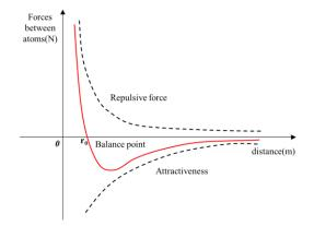
Figure 2. Atomic force-distance curve.
