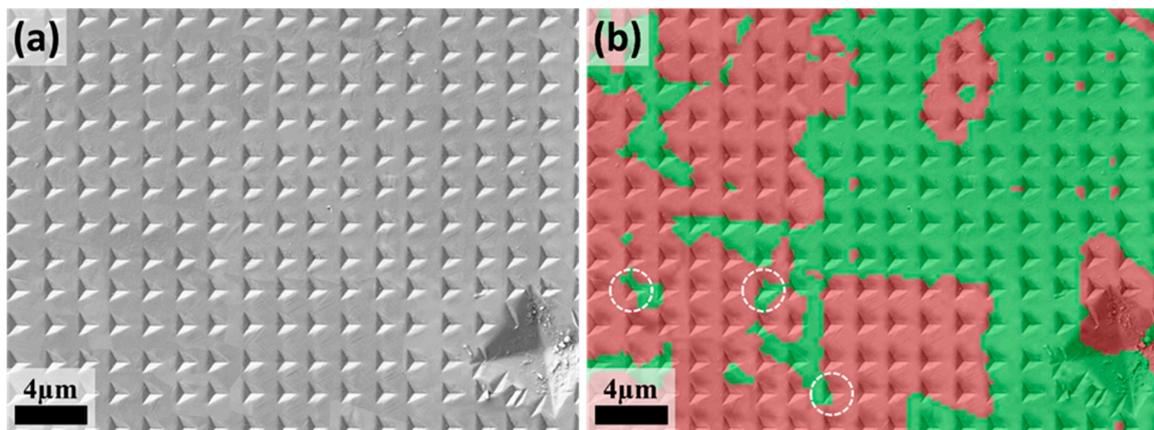
**Figure 6.** (a) Field emission scanning electron microscope (FESEM) micrograph of a region of the indented surface. (b) Phase map of the same region overlaid with the original micrograph.
