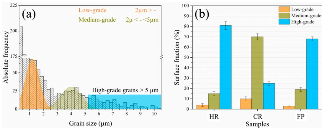
**Figure 4.** (a) Grain size histogram for HR sample, with 250 nm of bin size, computed from at least 2000 counted grains. (b) Surface fraction occupied by grains with different size ranges for all the studied samples.
