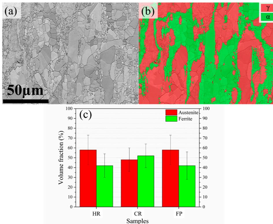
**Figure 3.** (a) Microstructure of the hot rolled (HR) sample illustrated by IQ; (b) phase map which illustrates the surface fraction of the  $\gamma$  and  $\alpha$  phases; and (c) volume fractions of both constitutive phases for all the studied samples.
