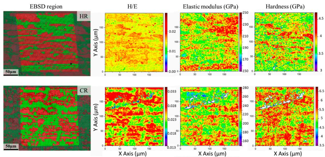
**Figure 7.** Electron backscatter diffraction (EBSD) maps of indented surfaces and corresponding cartography maps of indicated region for HR and CR samples.
