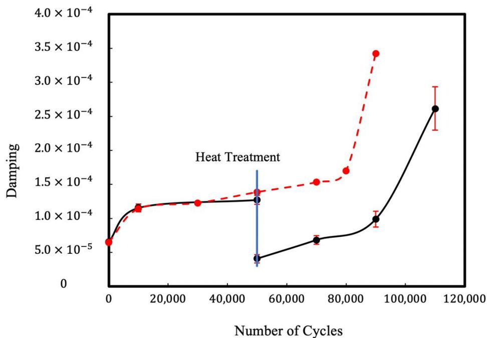
**Figure 5.** Evolution of damping for an SS316 specimen versus the number of cycles with the load frequency of 20 Hz and stress amplitude of 432 MPa halted and heat-treated at the temperature of 600 °C, at its half-life (50 k cycles). Dashed line results are the damping values of an untreated (as-received) specimen as a benchmark.
