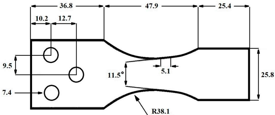
Figure 2. Schematic of the dog-bone flat SS316 specimen (all dimensions are in millimeters).
