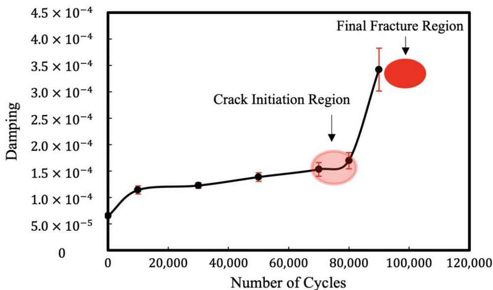
**Figure 4.** Evolution of damping versus the number of cycles for an SS316 specimen at the frequency of 20 Hz and stress level of 432 MPa.
