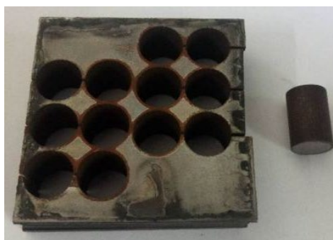
Figure 2. Appearance of billet and specimen used for the hot compression test.
