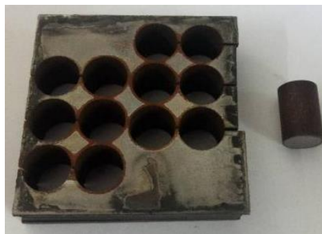
Figure 2. Appearance of billet and specimen used for the hot compression test.
