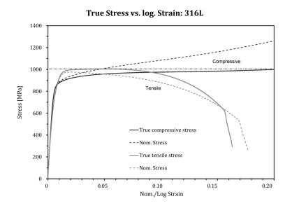
Figure 3. Test data displayed as True Stress vs. Logarithmic Strain.
