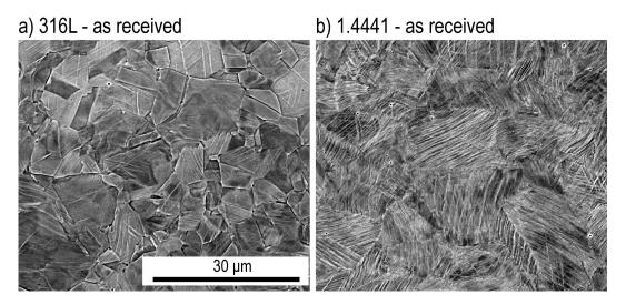
**Figure 5.** Microscopy using backscattered electrons reveals the microstructures in the as-received state of (**a**) 316L and (**b**) 1.4441.
