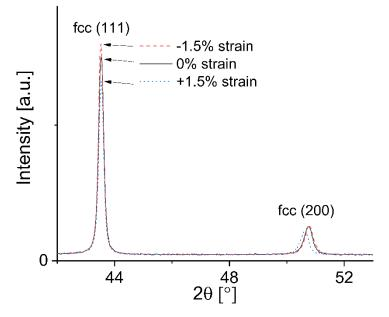
**Figure 7.** XRD measurements of 316L taken at 0% strain, +1.5% and -1.5% strain. The normal vector of the diffraction planes is aligned parallel to the loading direction.
