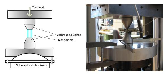
**Figure 1.** Schematic view of the mechanical setup (**left**) and installation with prepared sample in the test machine (**right**), with large plates adjusted and fixed in parallel.
