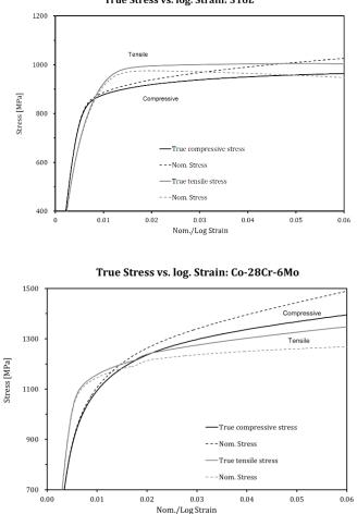
Figure 4. Asymmetry in steel 316L (top) and Co-28Cr-6Mo (bottom).
