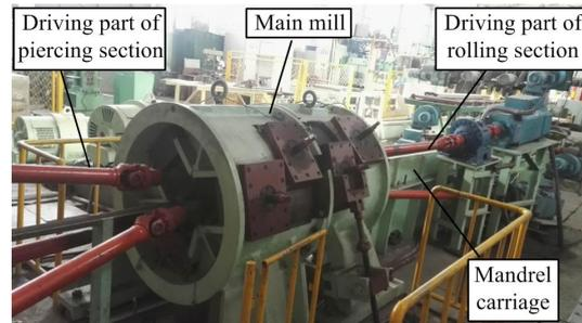
**Figure 2.** TSR testing mill.
