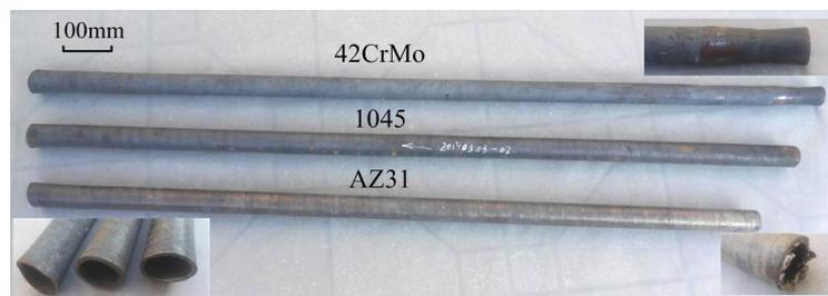
**Figure 9.** Seamless tubes produced in the TSR testing mill.
