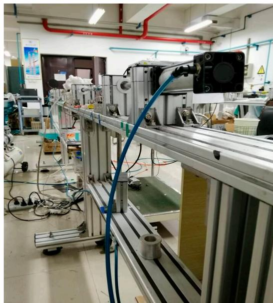
Figure 5. Hopkinson pressure bar experimental device.
