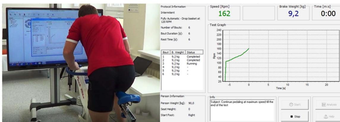
**Figure 1.** Testing configuration with visual feedback appearing 2 meters in front of the cycle ergometer. The participants were instructed to look at the revolution-time curve, which was adjusted to their field of vision during specific warm-up.
