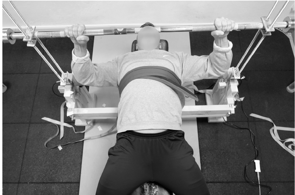
Figure 1. The testing setup. The participant's test positions for the bench press (push) and supine row (pull) are depicted. For the supine bench row, the upper body was secured against the bench by a heavy-duty Velcro fixation belt. This custom-built setup has previously been described and validated for use in elite throwers [16].
