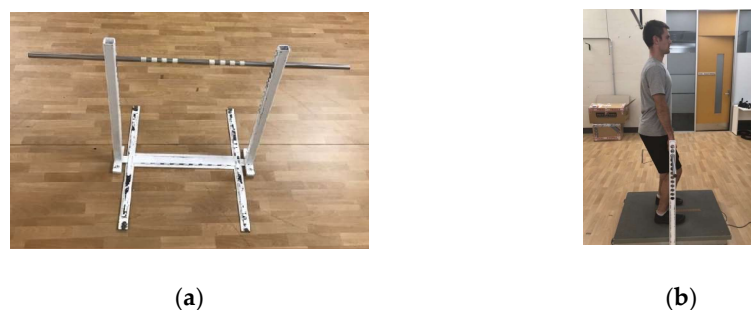
Figure 1. Set-up for Isometric Mid-Thigh Pull testing: (a) specialised portable rig; (b) participant positioning [23].
