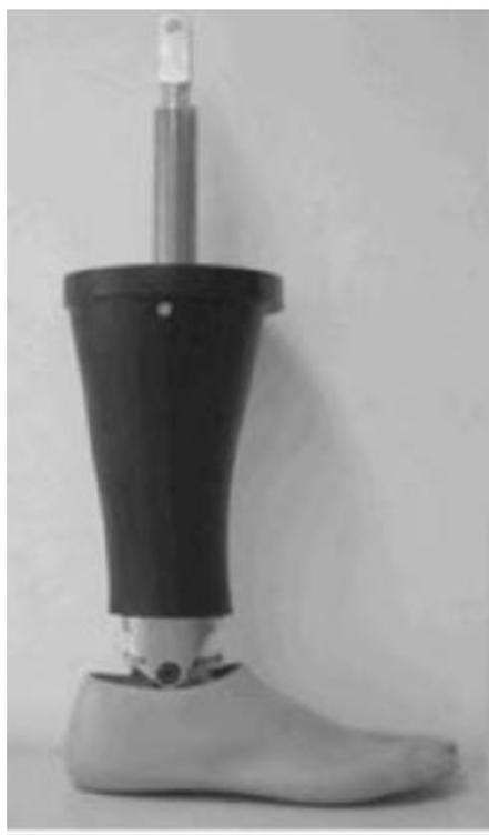
**Figure 12.** Ski-boot test bench (from reference [41]).
