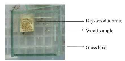
Figure 1. Glass box of dry-wood termite test [3].
