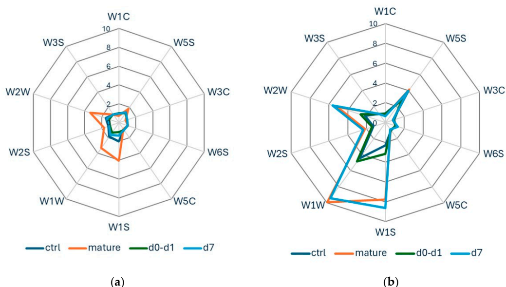
Figure 2. Radar plots of e-nose sensor response values for (a) peaches after infestation by B. zonata , (b) peaches after infestation by C. capitata , stored at 20 °C, and their corresponding control samples.
