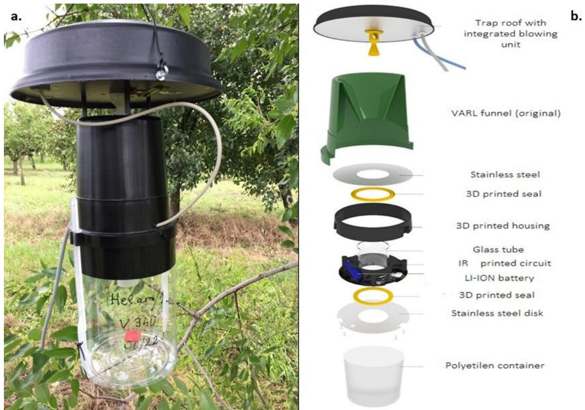
**Figure 1.** ZooLog VARL probe prototype in the field (a) and its 3D schematic diagram (b). The probe was built to detect flying insects, mostly pest moths and other lepidopteran pests. The probe was baited with a pheromone lure of the target insect; insects dropping through the funnels into the catch container could not escape. An infrared sensor-ring detects the individuals, and a blow-off system directs the flying insects toward the catch container. For further details, see Supplement S2.
