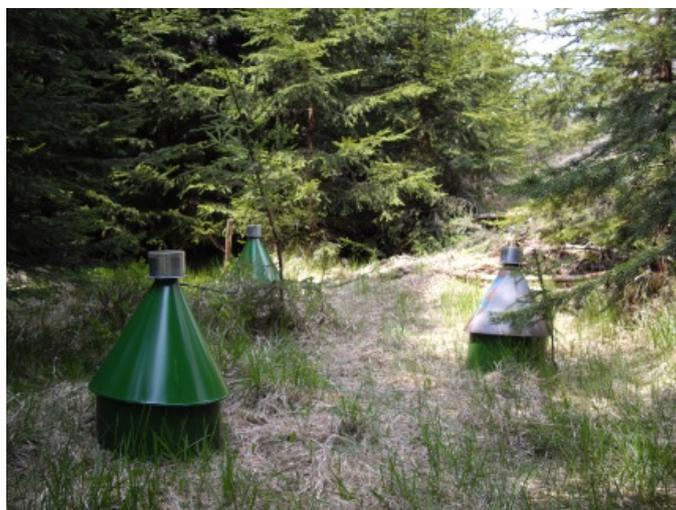
**Figure 2.** The soil photoelectors that were used to collect thrips.
