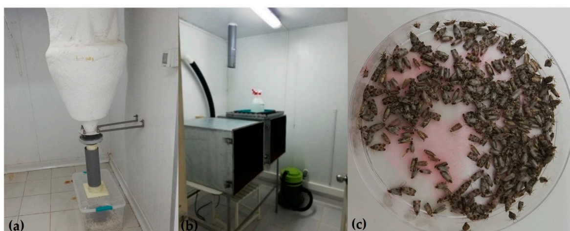
Figure 2. (a) Cyclone collection trap mounted in a cold room with collection box to hold moths immobilized by the cold. (b) Moth eclosion cabinets fitted with a fiber optic UV light and PVC ductwork vacuum system leading to the cyclone trap. (c) Irradiated EGVM moths marked with Dayglo™ fluorescent powder in Petri plate for release.
