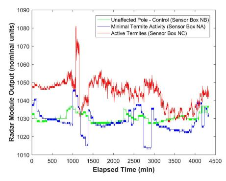
Figure 15. Radar response for three poles installed in the field in the Northern Territory.
