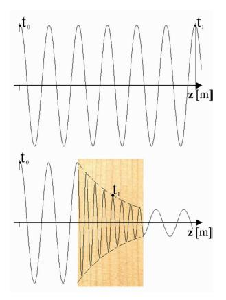
**Figure 1.** Propagation of microwave energy through air or open space (**top**) and through wood (**bottom**) [18].
