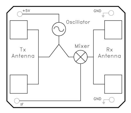
Figure 7. Block diagram for HB100 radar module.
