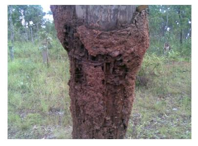
Figure 10. Extracted untreated pole showing active Mastotermes darwiniensis infestation.
