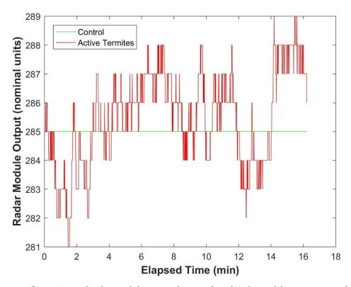
**Figure 13.** Comparison of radar module output for samples of timber at laboratory atmosphere equilibrium moisture content (EMC) with and without (Control) active termites present.
