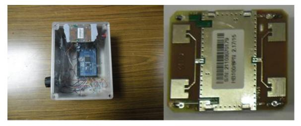
Figure 8. (Left) Sensor box with the HB100 radar module (right).
