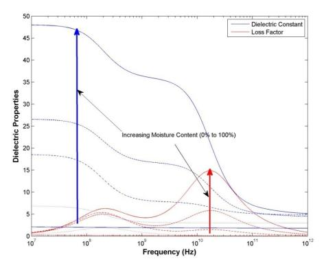
**Figure 2.** Dielectric properties of wood with the electric field parallel to the grain (density of  $600 \text{ kg m}^{-3}$ ) as a function of frequency and moisture content, based on data from Torgovnikov [7]
