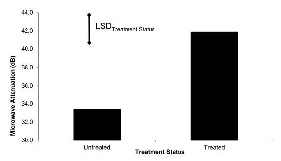
**Figure 11.** Mean microwave attenuation (dB) in sound Spotted Gum pole stubs as a function of timber treatment status.
