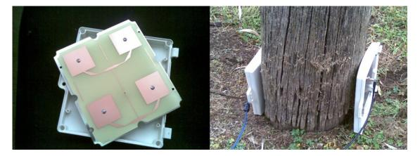
**Figure 6.** Microstrip antenna array (**left**) showing detail of the array and (**right**) showing the antennas in place for microwave testing of a power pole.
