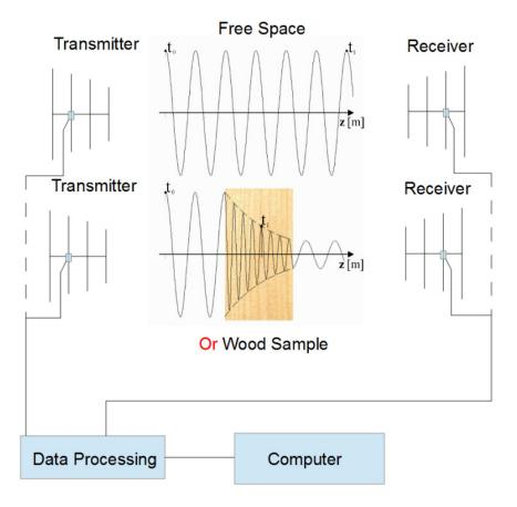
**Figure 5.** Schematic diagram of the sensor system for the microwave detection of termites and decay in wood with the wave pattern for open space/air shown at the top and the wave pattern for passing through wood shown below.
