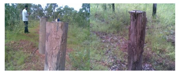
Figure 9. Untreated poles showing varying degrees of termite attack.
