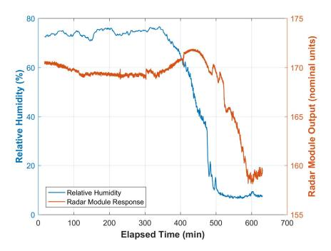
**Figure 14.** Output from a HB100 radar module, applied to a wooden sample block (30 mm by 30 mm by 200 mm), in response to changing external humidity.
