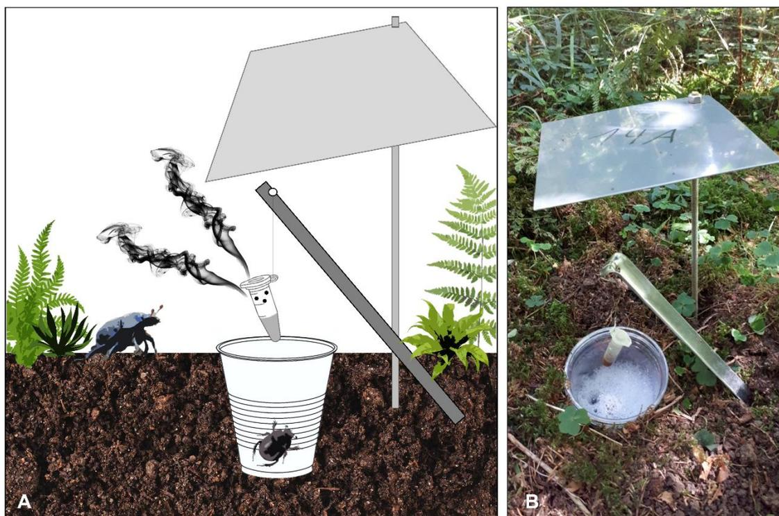
**Figure 1.** (A) Graphic illustration of a pitfall trap with bait (treatment) in a perforated Eppendorf tube used in the field assays and (B) the corresponding setup as an original image.
